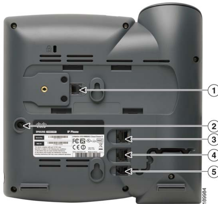
Figure 1 Cisco SPA 525G/525G2 IP Phone Connections
